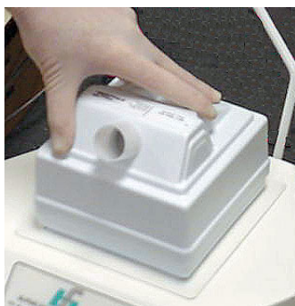
Figure C-9 Seating the new filter
