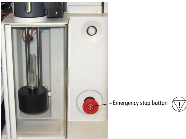
Figure 1-23 Emergency stop button
