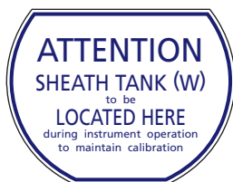
Figure 4-6 Sheath tank location label
